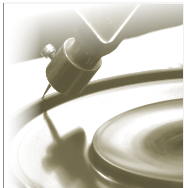
Trimming of oil seal
